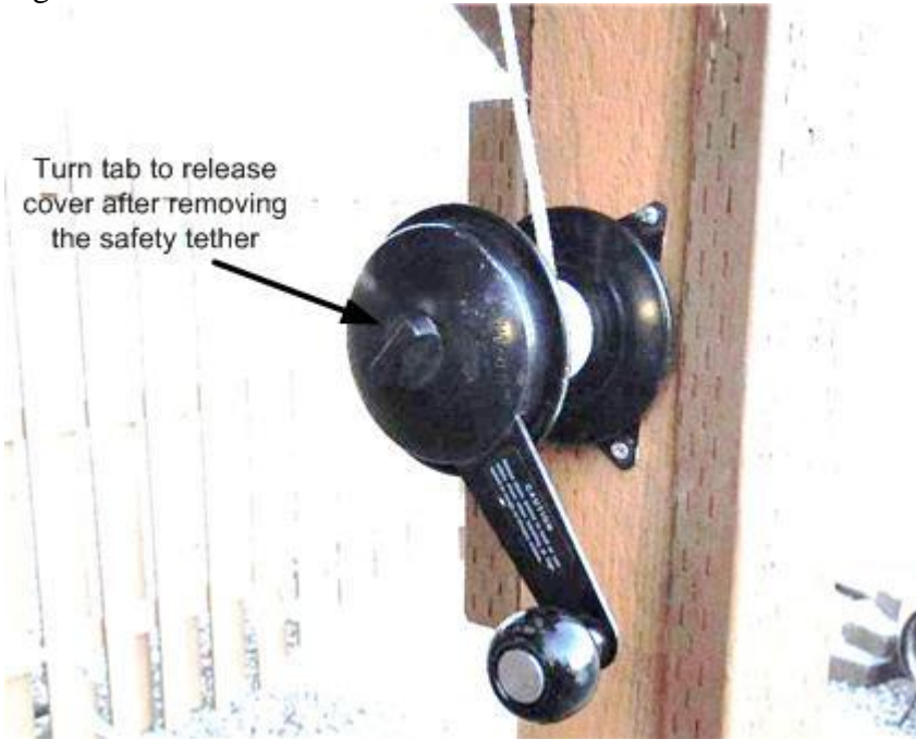
Figure 5. Cover is raised by turning the crank. Cover is released by turning the tab.
